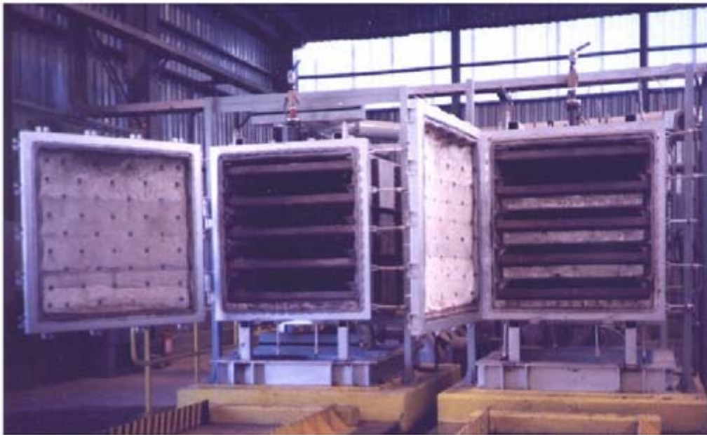
Interior of 30 cubic foot capacity retorts shown during loading.
